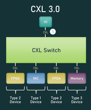
1 Each host's root port can connect to more than one device type
