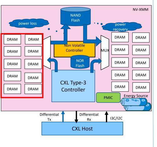
Non-volatile media based (like NVDIMM-P or Intel Optane™ DIMM)
