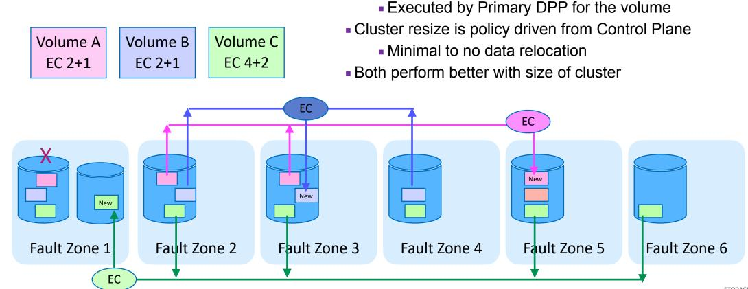
Rebuild each volume impacted by a failure (e.g. SSD)
