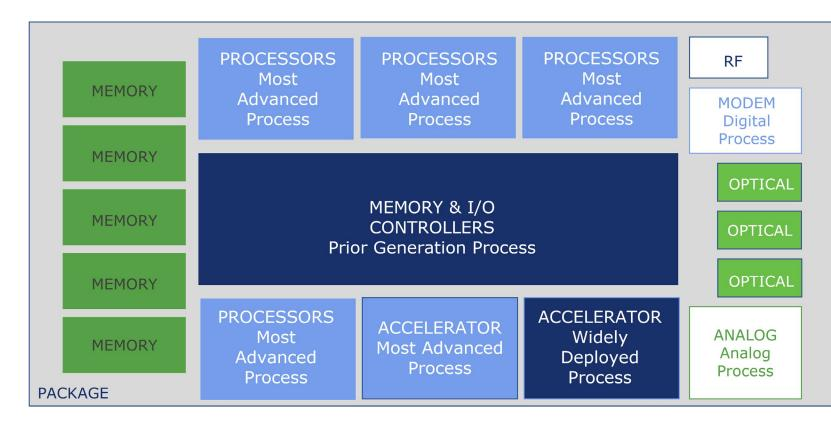
SoC Package level construction for wide range of usages from Hand-held to high-end servers
