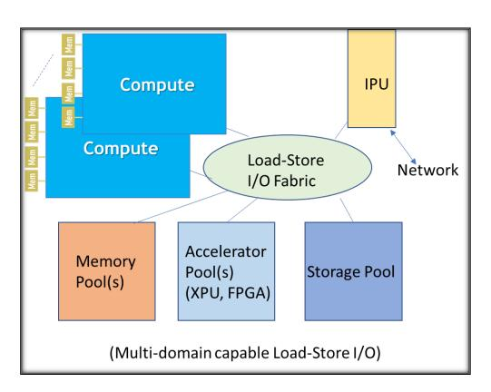
Vision: Load-Store I/O (CXL) as the fabric across the Pod providing lowlatency and high bandwidth resource pooling/sharing as well as message passing.
