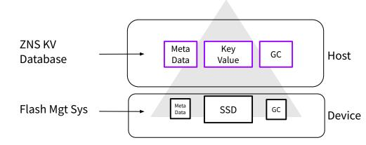
Simplify the device Flash management system to reduce the amount of metadata
