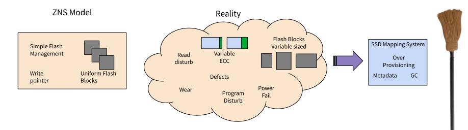
The 'hope' is that SSD Mapping system GC is close to 0 and that the Overprovisioning can be minimized...
