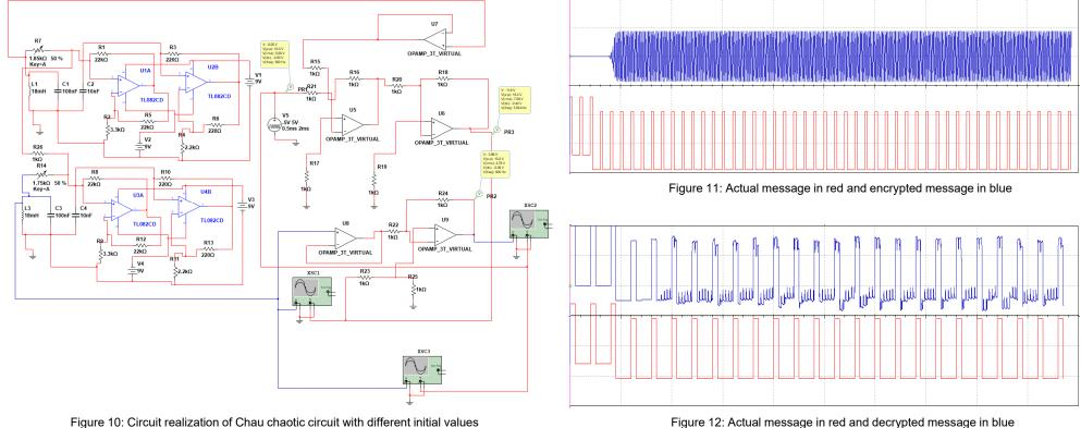
Figure 10: Circuit realization of Chau chaotic circuit with different initial values
