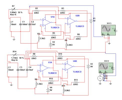
Figure 6: Circuit realization of Chau chaotic circuit
