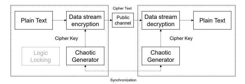
Figure 5: High level architecture of chaotic cryptography
