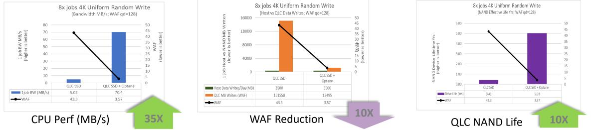
Single job QLC read BW is only 142MiB/s, cannot meet 250MiB/s target; Single job O+Q write BW is 163MiB/s, 18 times of QLC BW of 9.05MiB/s, while WAF is 3.54, only 8.7% of QLC WAF of 40.8.
