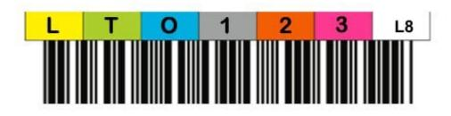
Barcode with volume serial number, generation, and type of cartridge
