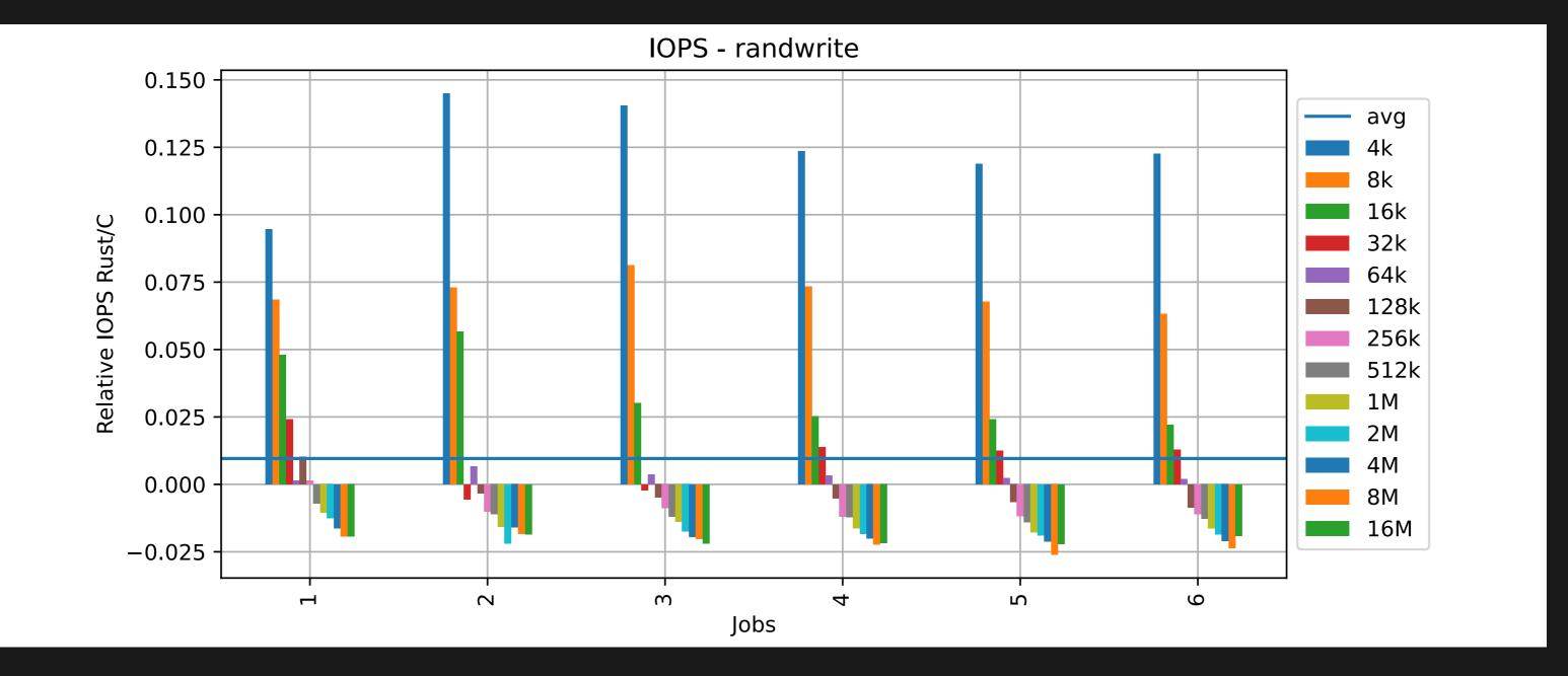
Intel Alder Lake workstation (i5-12600). 60s fio runs on bare metal, pinned workers, io\_uring, bs 4k to 1M -> QD 128, bs >= 2M -> QD 64, batch submit/complete -> 16.
