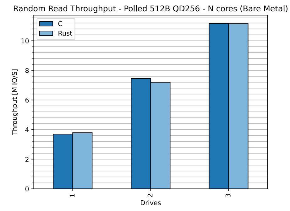
AMD EPYC 7313 3x INTEL P5800x 16GT/s x4 7.88 GB/s (PCIe 4), DATA FROM RUST/C NVME ON LINUX 6.1
