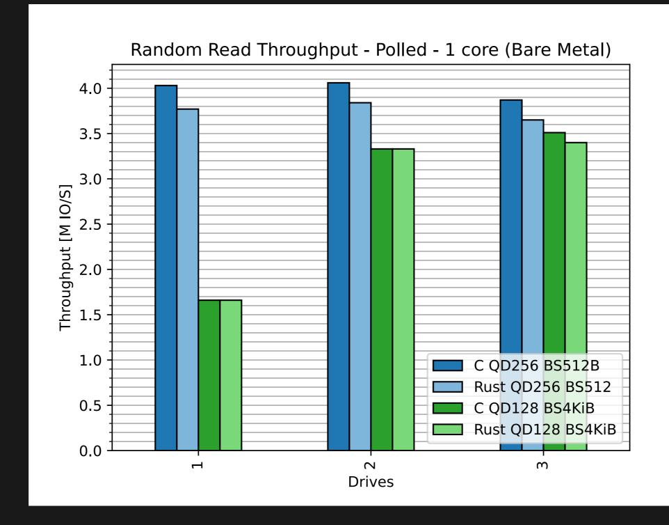
AMD EPYC 7313 3x INTEL P5800x 16GT/s x4 7.88 GB/s (PCIe 4), DATA FROM RUST/C NVME ON LINUX 6.1
