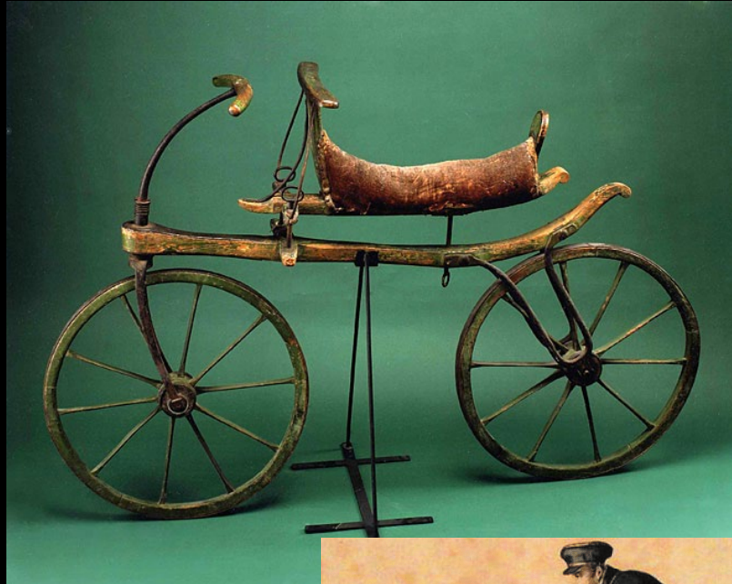
Draisine (Running machine), 1817: the 1 st bicycle in record
