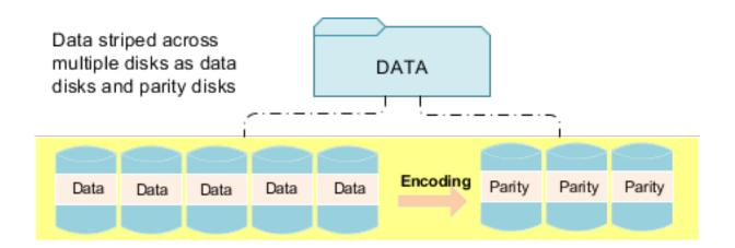
Data protection algorithms designed for HDD
