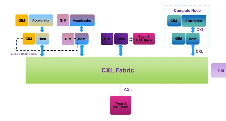
Host to Fabric-Attached Memory (FAM) communication with Global Integrated Memory (GIM)
